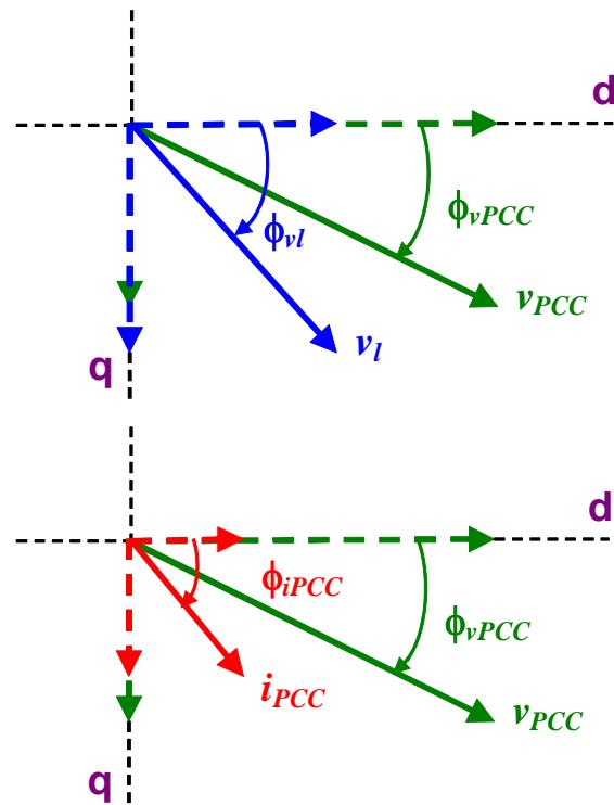
$$\phi_{vPCC} := \operatorname{atan}\left(\frac{v_{iq} - R_i \cdot i_{iq} - w_s \cdot L_i \cdot i_{id}}{v_{id} - R_i \cdot i_{id} + w_s \cdot L_i \cdot i_{iq}}\right) \cdot \frac{180}{\pi} \quad \phi_{vPCC} = -1.596$$
